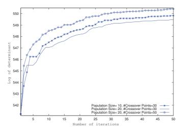
Figure 2: Coupled Fedorov genetic algorithm: case of Hermite polynomial of degree p=4, with M=6 variables and N=420 experiments.
